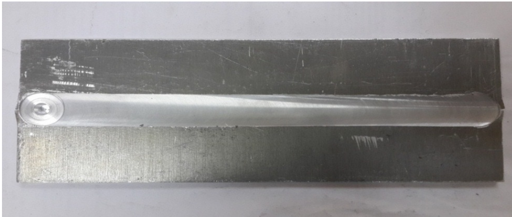
Fig. 4. Friction Stir welded AA6082 plate
