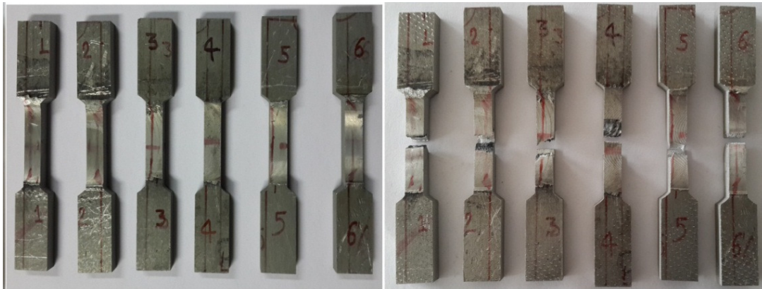
Fig. 5. Tensile test specimen before and after the test
